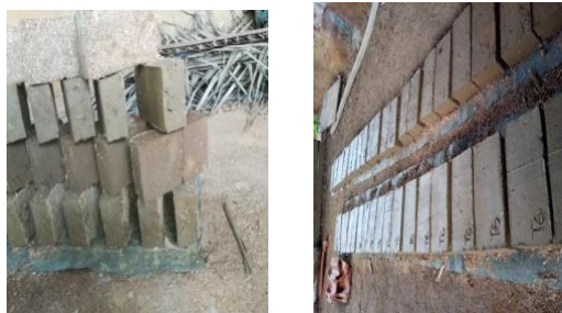
Figure 1. Produced Bricks Stacked for Drying
