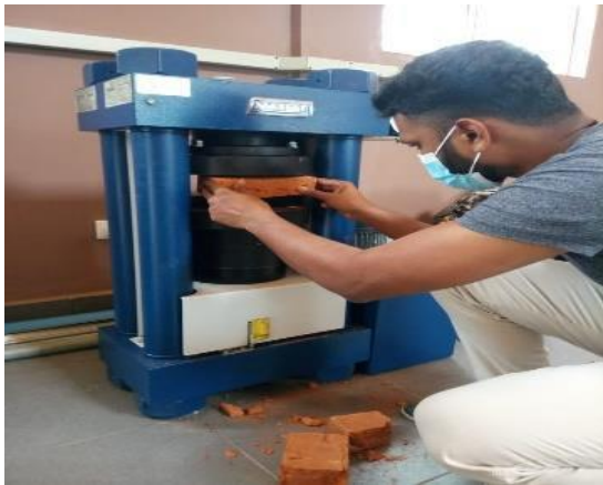
Figure 2. Monitoring the Compressive Strength of Bricks
